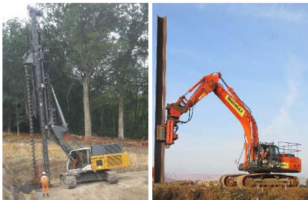
Auger (drill) rig
