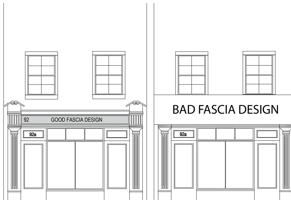
Figure 10. Poor fascia sign sizes and design can overbear the shop front and obscure architectural detailing. Fascia signs should seek to work with the building and existing features.
