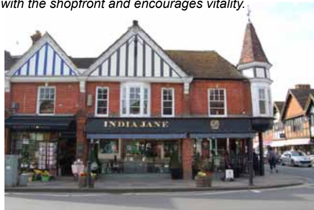
Figure 7. High Street, Haslemere: The large modern shop window here is a good example as it respects the proportions and detailing of the building. The retention of the brick pilaster in line with the end of the gable provides visual strength to the shopfront. The fascia could have been split in line with the retractable awnings to retain visual rhythm of the original shopfronts.
