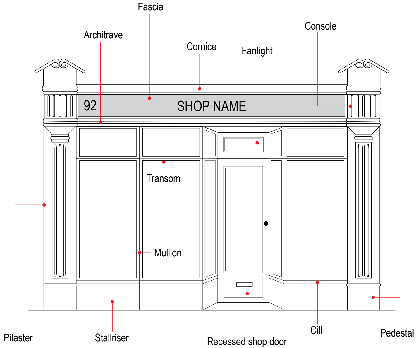
Figure 1: This figure identifies the different elements which make up a traditional shopfront. Within modern shopfronts, some of these elements may not be used.
