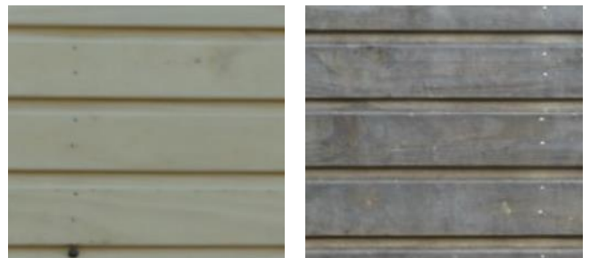
Accoya cladding: left- newly installed right - after weathering of the timber Source: Accoya Technical Leaflet Weathering V08.15-3.
